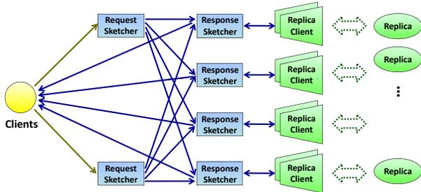
Figure 4: Scaling out Prophecy using multiple sketchers.
