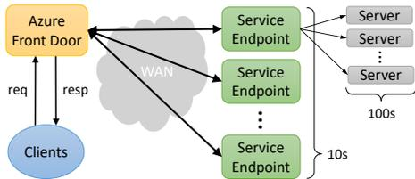
Figure 6: Hierarchical architecture of Azure Front Door.
